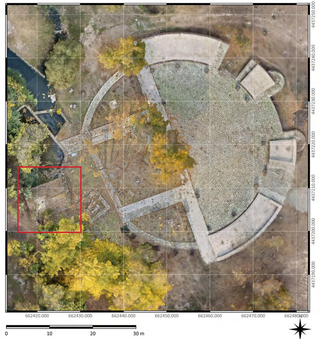
Fig. 4. Georeferenced ortho-image of the mosque and the spring sources extracted from the textured 3D scan (Iconem 2021)
