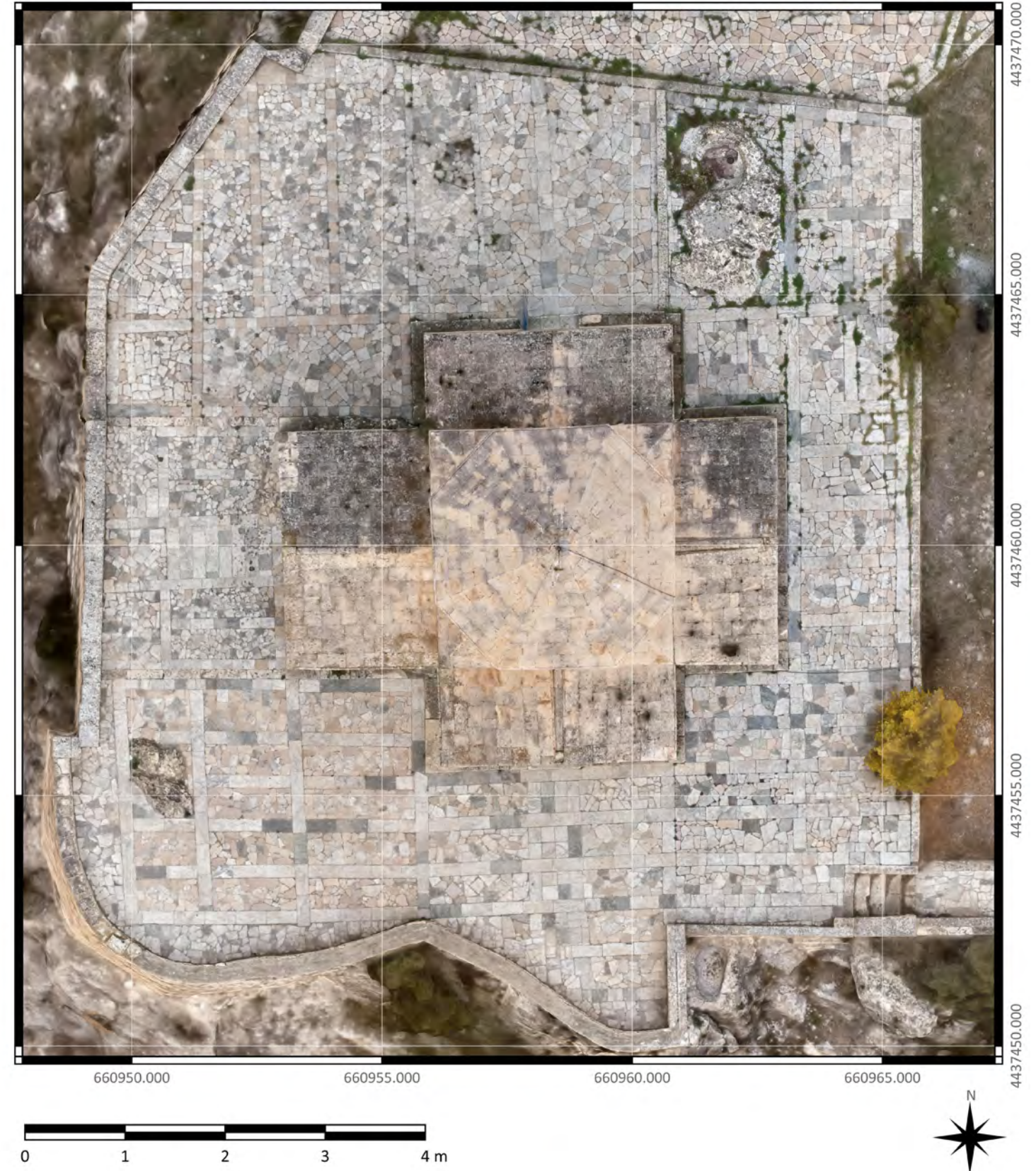
Fig. 2. Georeferenced ortho-image of Vankasar church extracted from the textured 3D scan (Iconem 2021)
