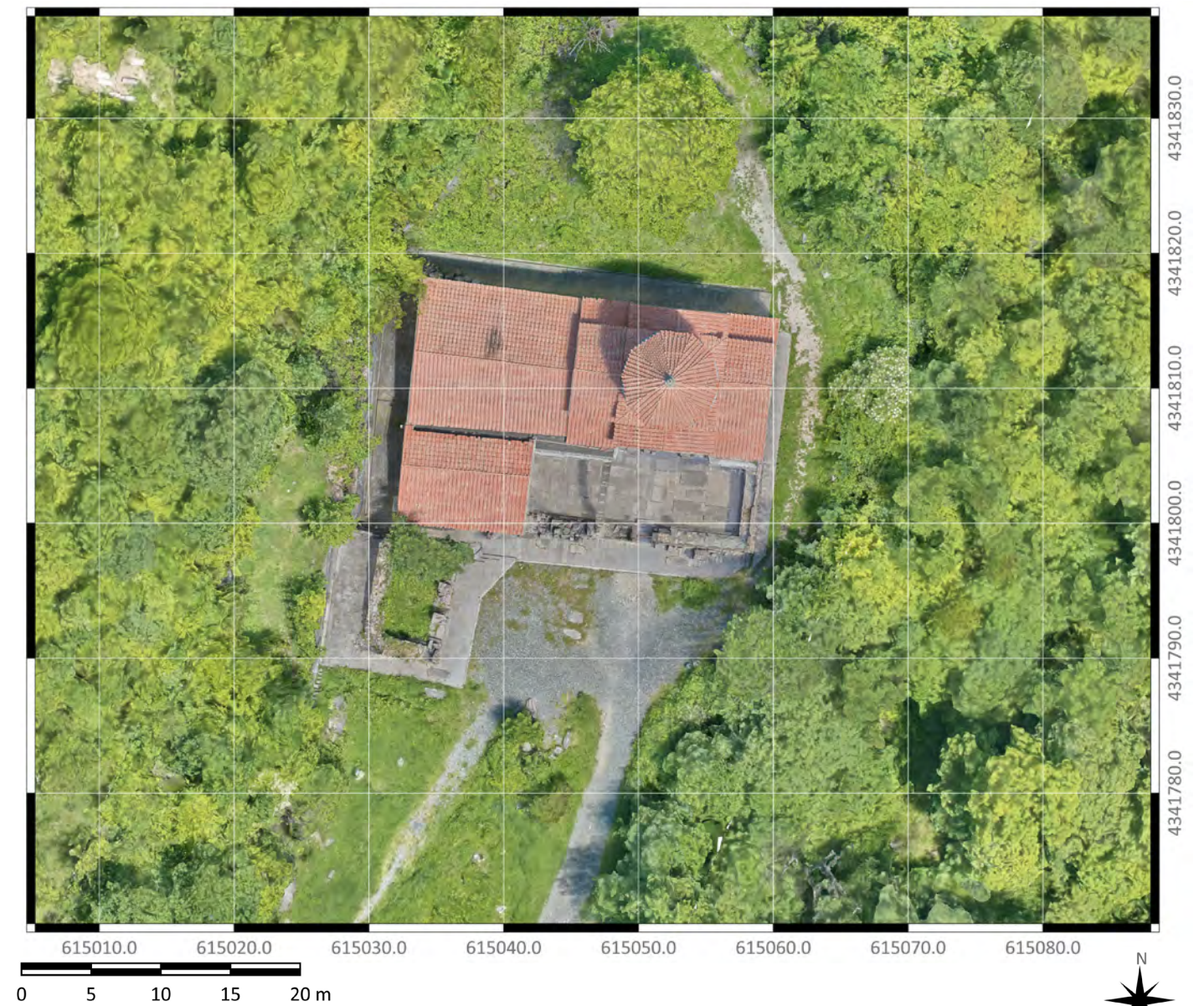
Fig. 2. Georeferenced ortho-image of the monastery of Vahanavank extracted from the textured 3D scan (Iconem 2021)
