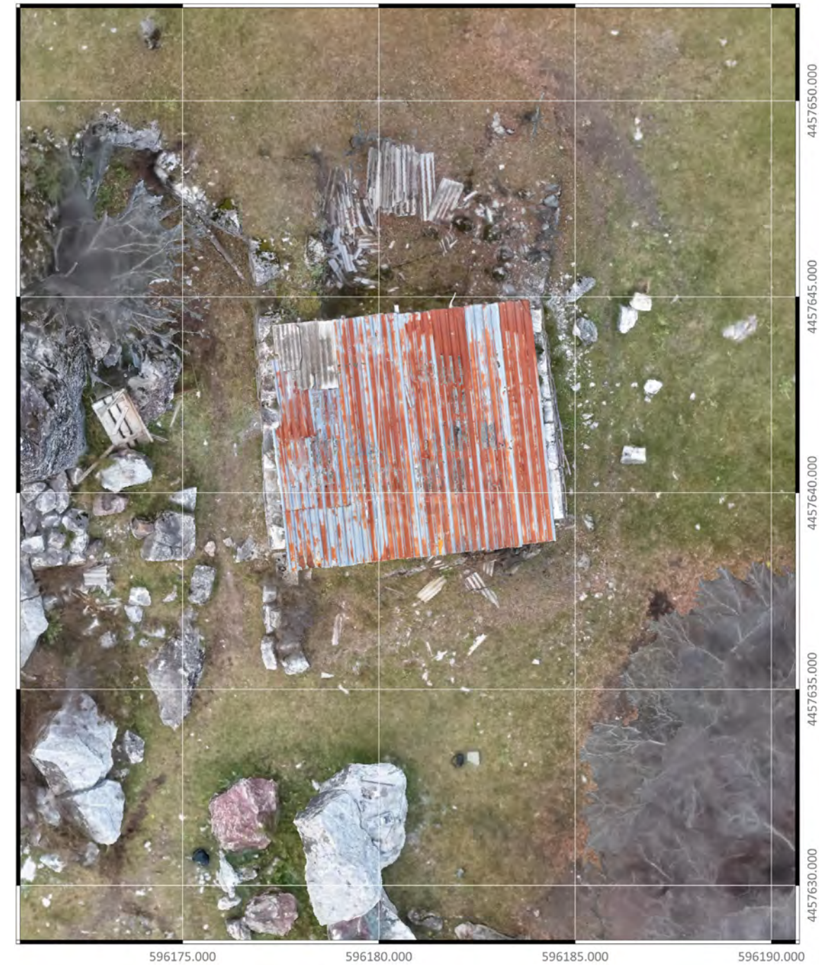
Fig. 2 Georeferenced ortho-image of Takyaghaya church extracted from the textured 3D scan (Iconem 2021)
