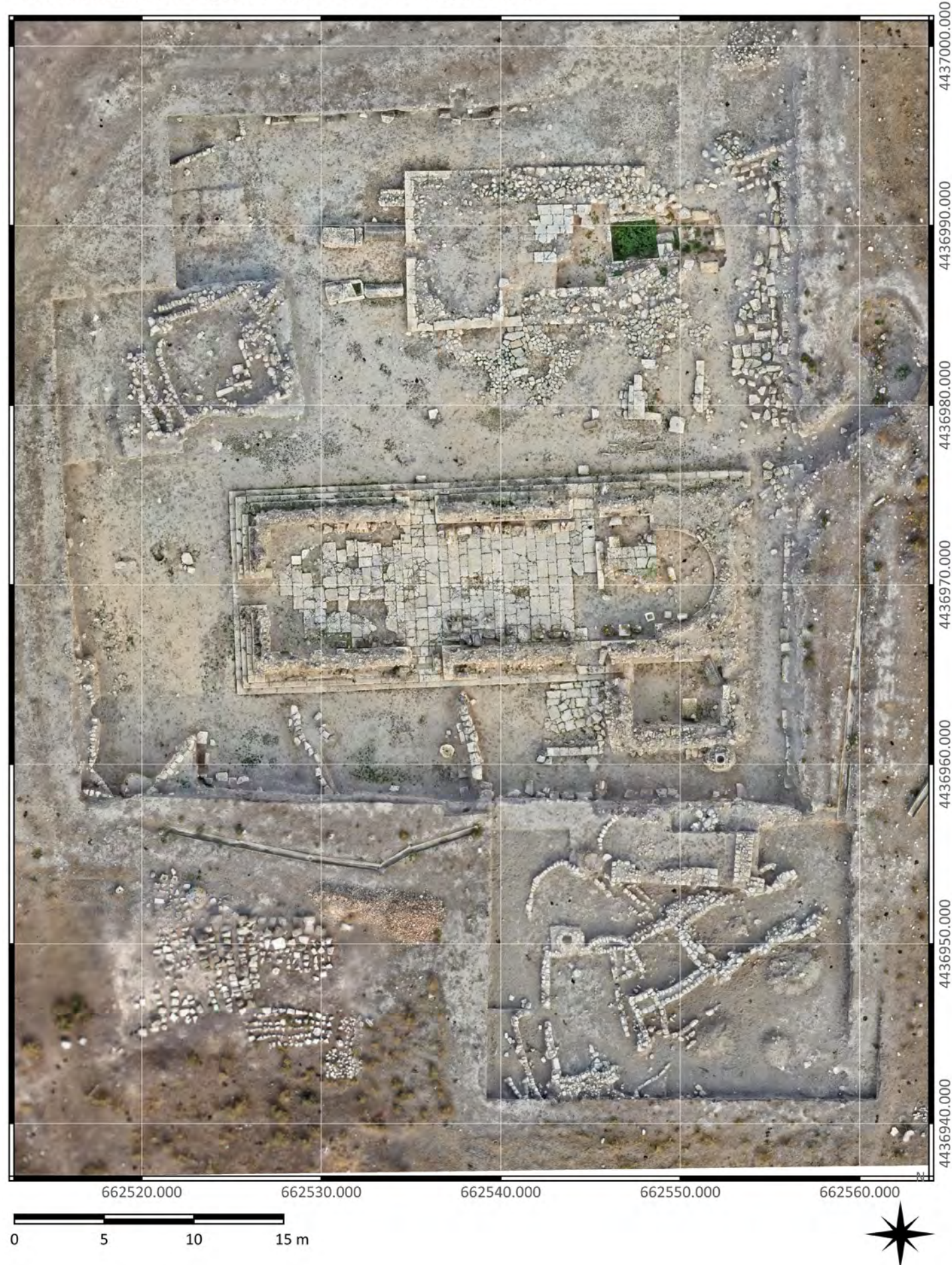
Fig. 3. Georeferenced ortho-image of the early Christian square extracted from the textured 3D scan (Iconem 2021)
